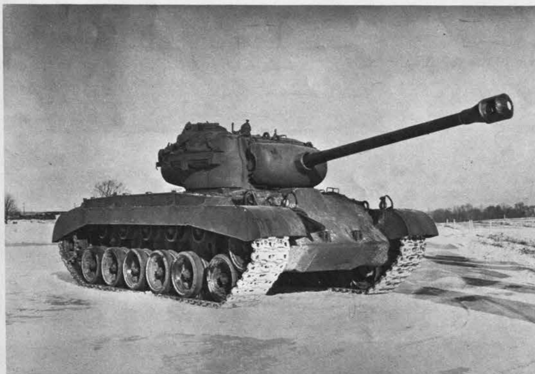
Newest and most powerful U.S. tank, the Pershing M-26 has widely used suspension called the torsion bar, often erroneously called Christie. Like the Stalin, it has its driving sprocket at the rear.
